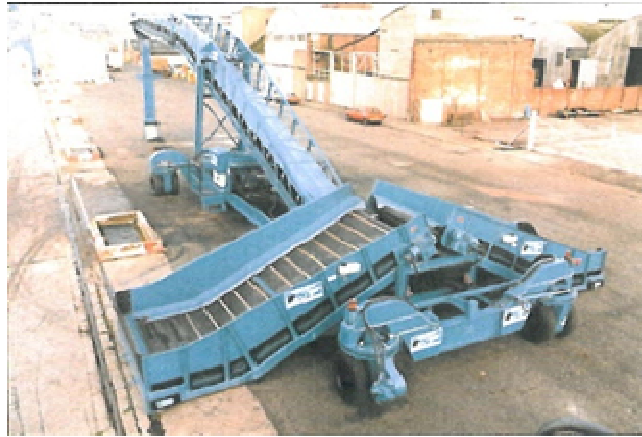
Figure 3-53: Typical Mobile Shiploader
